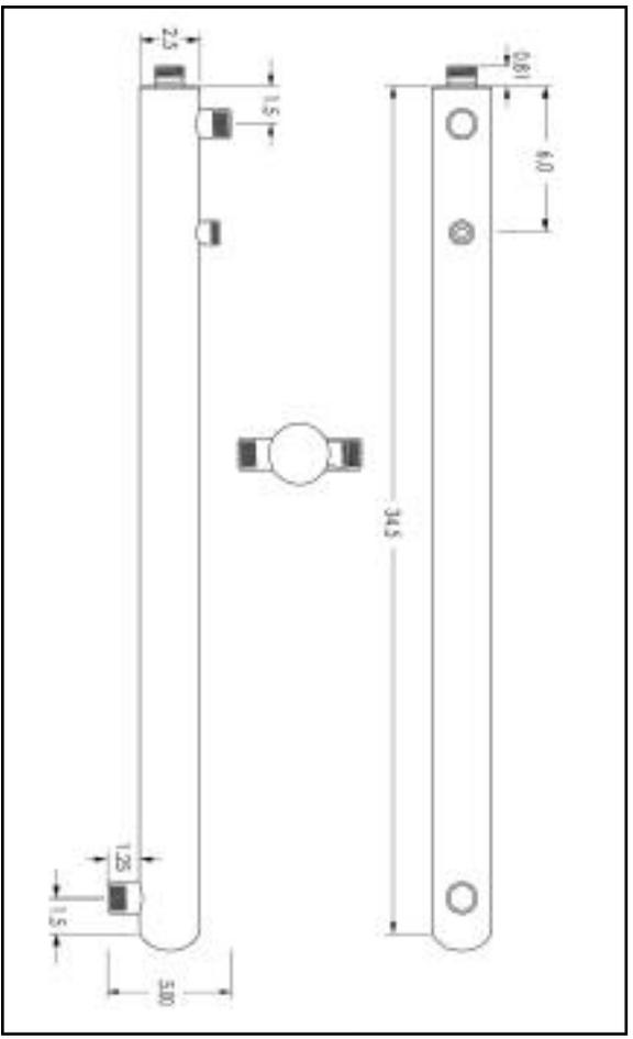
**UV Dosage & System Schematic – All Measurements in inches (1" = 25.4 mm)
