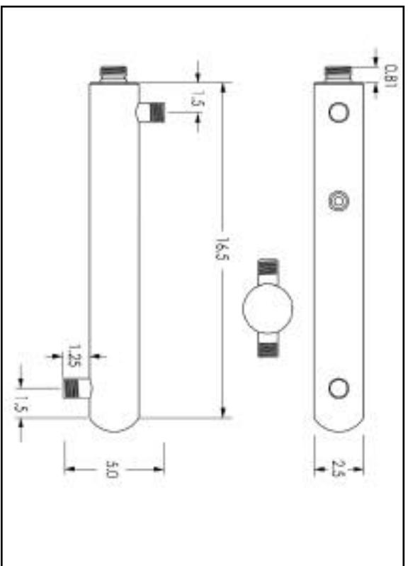
**UV Dosage & System Schematic – All Measurements in inches (1" = 25.4 mm)
